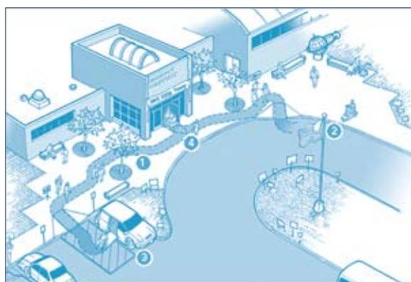
Image 9.12: An accessible entrance to a polling place with accessible parking and an accessible drop-off area.
